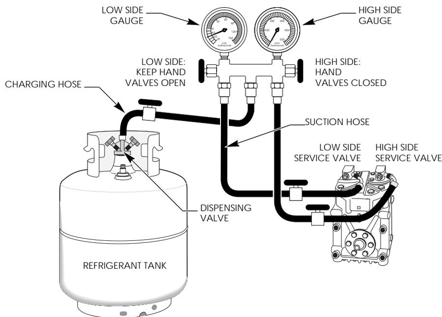
5. Check the sight glass when you have added nearly the specified amount of refrigerant. Keep adding refrigerant until the sight glass clears or you have added the specified refrigerant charge. Use an oil injector to replace oil drained from the system. Remember, a large leak may have resulted in nearly all the lubricant being lost.
