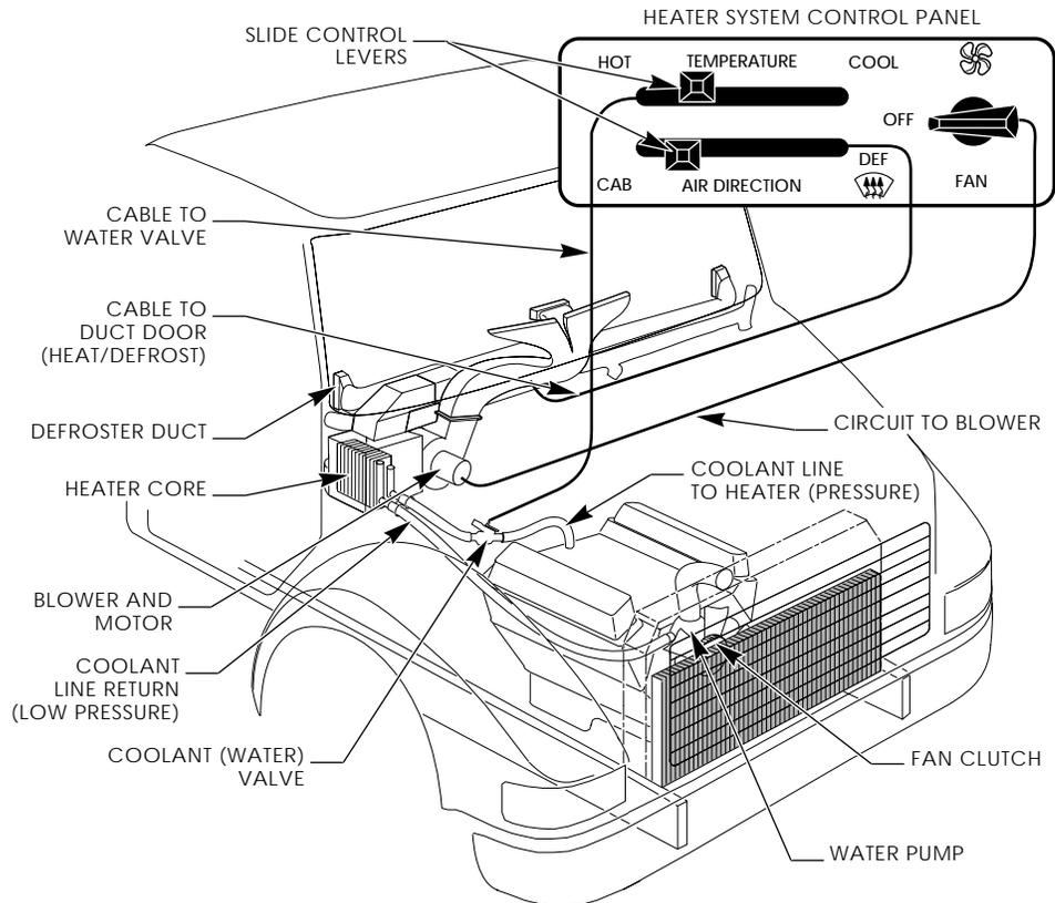
A water valve is the primary control for a basic heater system. When the valve is open, hot engine coolant flows through the heater core and back to the engine. The driver can adjust the control to modulate coolant flow through the heater core.
