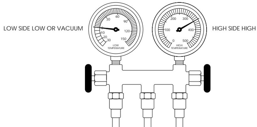
**Tip:** Air from vents in the cab is only slightly cool. The expansion valve body is frosted or sweating.
