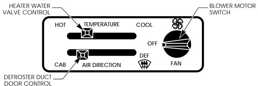
When you turn the system on, the water valve opens to allow hot engine coolant to flow through the heater core. The blower motor circulates cab air through the heater core to warm the air. Water valves may be cable or air operated. Figure 3-8 illustrates both types.
