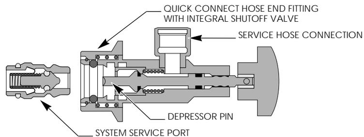
VALVE ASSEMBLED TO SERVICE PORT WITH VALVE IN THE OPEN POSITION
