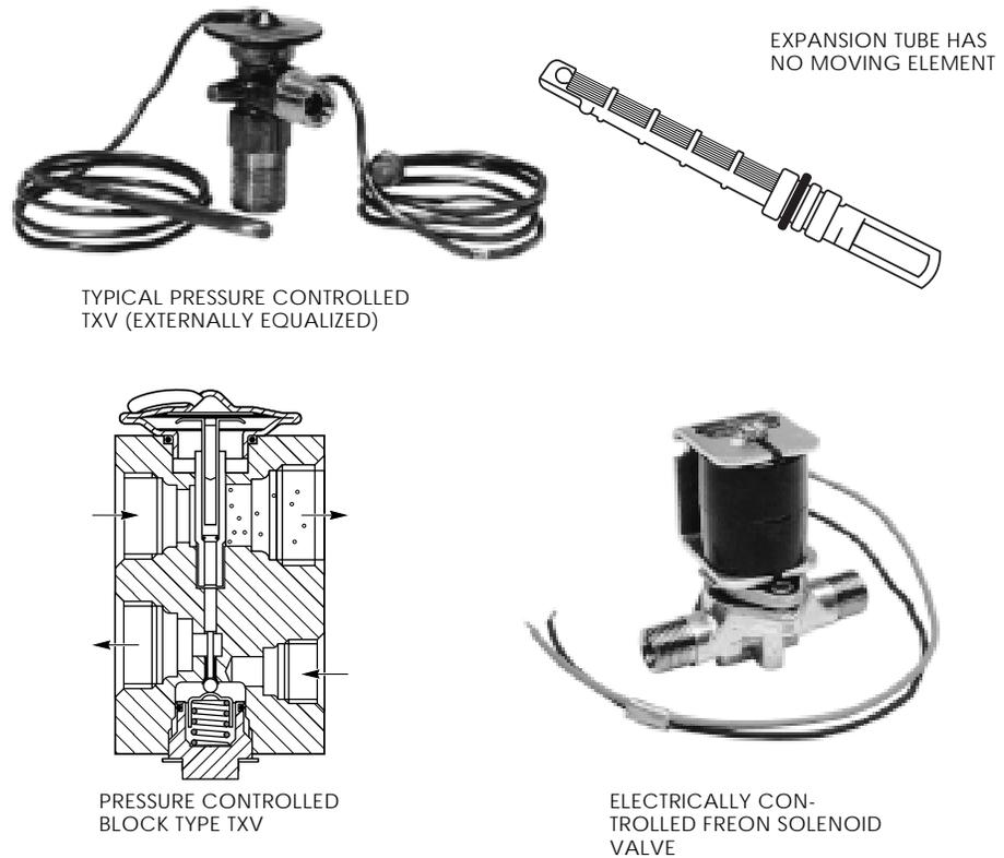
These controls are designed to meter refrigerant flow through the evaporator coil. Thermostat and compressor clutch function are independent of these refrigerant flow control devices.
