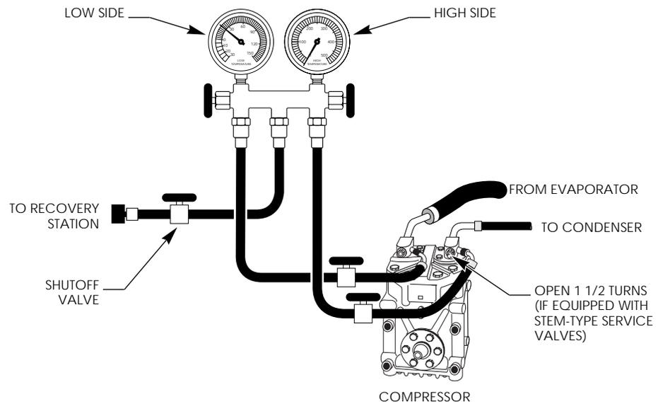
**Note:** The manifold gauges read system pressure when the hand valves are closed if the hose end valves, and the stem type service valves (if included) are open.
