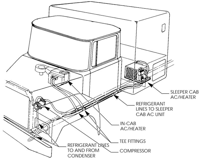
Engine intercooler designs often use the space in front of the radiator where an AC condenser would normally be mounted. A roof mount AC system condenser may be the solution. In some cases, there is space to install the condenser below the intercooler. Figure 11-9 illustrates how an AC system design takes advantage of space below the intercooler for condenser installation.
