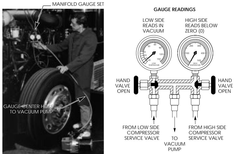
2. Start the vacuum pump and open both the hand valves on the manifold all the way. Run the pump for five minutes, then close the hand valves and shut off the pump.
