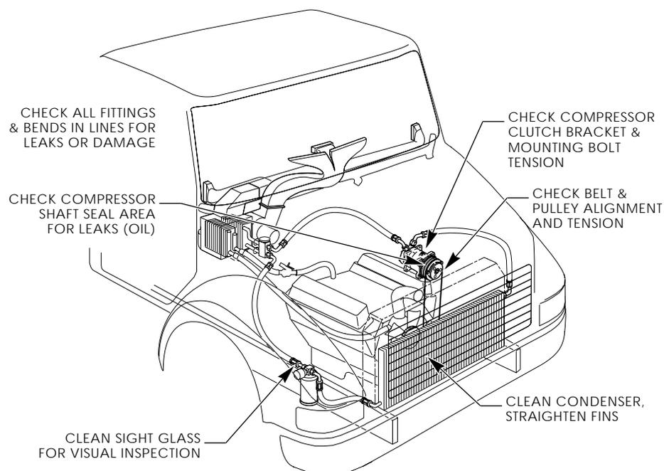
**A. Condenser** – Is it free of leaves, bugs, bird feathers or mud? The condenser must be relatively clean to work well as a heat exchanger. How you clean the condenser depends on where it is mounted. The condenser fin comb, air hose and nozzle, or soap and water may be used. Where possible, check condenser mounting bolts or screws and tighten them if necessary.
