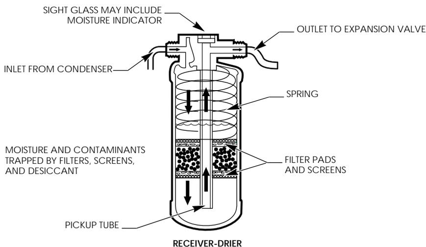
**Note:** Moisture (water) or particles can cause system malfunctions and corrosion. They can block the natural flow of refrigerant at the expansion valve. Moisture can change state there and form ice. It may also mix with the other elements inside the system (refrigerant and the oil) to form acid.
