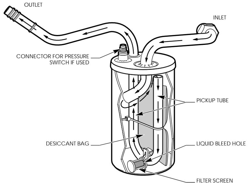
Most AC systems with an accumulator have a thermostat to control the clutch. The thermostat is usually positioned to sense refrigerant temperature between the evaporator outlet and the accumulator. Some AC systems with an accumulator have a pressure switch mounted on the accumulator to control the compressor clutch.
