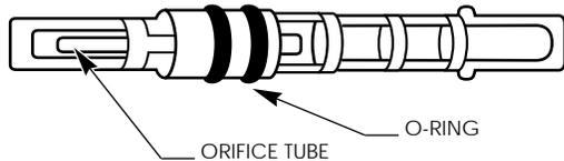
EXPANSION TUBES FIT INSIDE THE EVAPORATOR INLET FITTING
