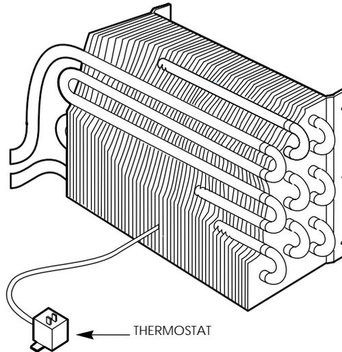
**Note:** Moisture in the air (humidity) condenses on the fins of the evaporator as water droplets which drain out of the evaporator through a drain hose. This action dehumidifies the air in the cab as part of system operation, and contributes to operator comfort.
