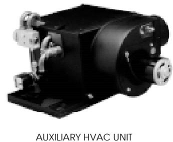
Sleeper cab AC system refrigerant flow is controlled by an electrically operated solenoid valve. The solenoid is wired to the control panel in the sleeper cab. When the operator turns on the bunk AC system, the solenoid valve opens to allow refrigerant to flow to the evaporator mounted under the bunk. With most installations the fan motor cycles on and off to control temperature. Figure 11-8 shows how the sleeper box and in cab AC units may be positioned and connected.
