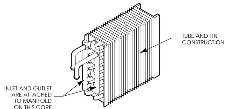
A large capacity heater core has more tubes and more fin area so that more coolant can circulate through the tubes and more air moves through the fins. The result is more heat energy transfer to the air in the cab.
