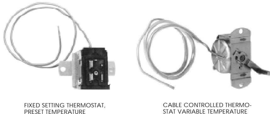
The thermostats shown have sealed capillary tubes that sense temperature. The capillary tubes contain a small amount of heat sensitive gas or liquid like R-12. System temperature variations raise and lower pressure in the sealed capillary tube. This pressure activates a switch inside the thermostat to open and close the electrical circuit to the clutch. These thermostats may sense temperature in the evaporator coil or at the evaporator outlet.
