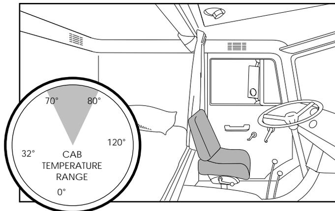
The ideal cab environment has a modest humidity level. The temperature should reach and then remain in the ideal range, 70 to 80 degrees. The cab should reach this temperature range after a few minutes of system operation with the windows closed. Air within the cab should be exchanged every few minutes to remove smoke, products of respiration and other odors.
