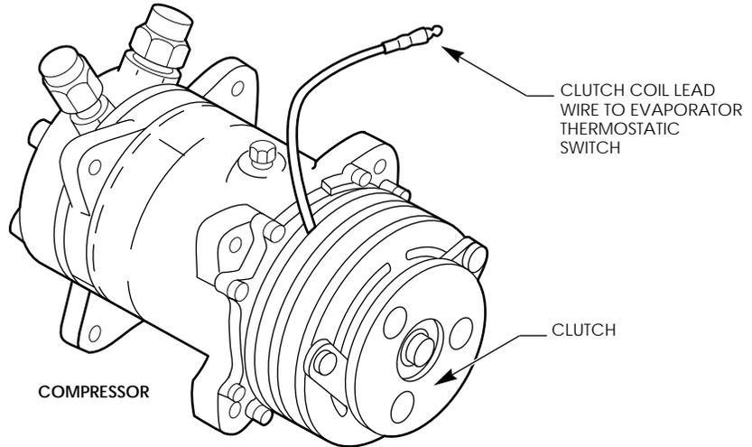
**Note:** In some systems (primarily GM systems) the clutch remains engaged to drive the compressor continuously during normal operation of the air conditioner. System pressure and refrigerant flow are controlled using suction throttling or POA valves at the outlet of the evaporator.
