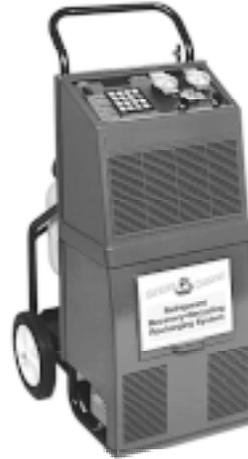
A full system recovery is not necessary when you service or replace a compressor with stem type service valves. These valves may be front seated to isolate the rest of the AC system from the compressor. The refrigerant stays in the system and only the refrigerant in the compressor is recovered, recycled and replaced.
